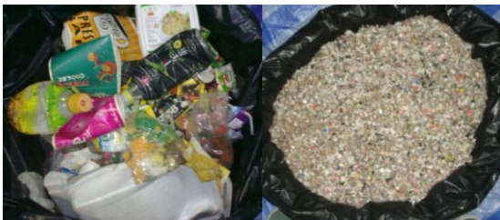
Fig. 4 Dry waste before cutting (left) and after cutting (right)
